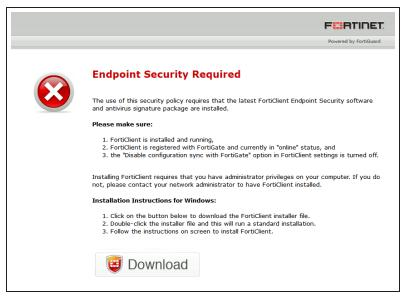
A download link is provided at the bottom of the page. When the user clicks on this link, the FortiGate responds with a download of the latest FortiClient software.
