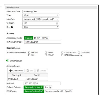
Create the VLAN interface for techdoc-200 and set up DHCP service.
